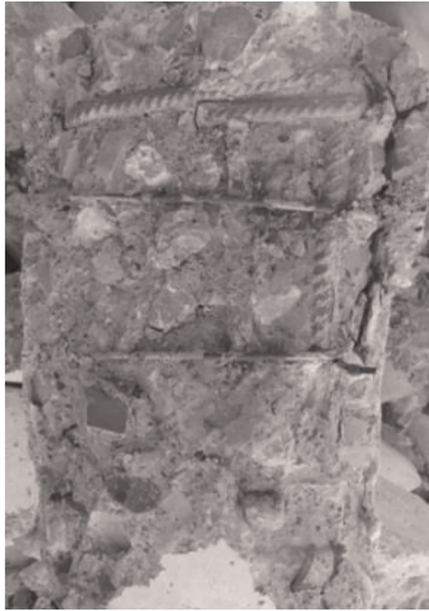
Figure 5. The fracture mechanism of the corroded reinforced rectangular specimens [13].
