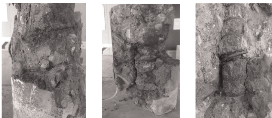
Figure 3. The fracture mechanism of the corroded reinforced cylindrical specimens [12].
