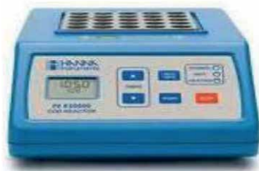
Figure 6. HANNA thermoreactor for heating water samples.
