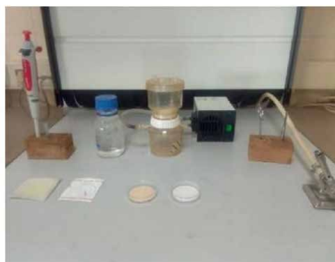
Figure 9. Equipment and consumables for the determination of bacteriological parameters. Top from left to right: The Pasteur pipette, bottle of physiological water, filtration device with an electric vacuum cleaner, a pair of scissors, and a Bunsen nozzle. Bottom from left to right: the filter membrane, the Petri dish containing culture media in cardboard [2].
