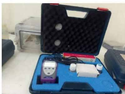
Figure 3. COND 70+ for measuring electrical conductivity and total dissolved solids.
