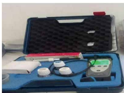
Figure 3. COND 70+ for measuring electrical conductivity and total dissolved solids.
