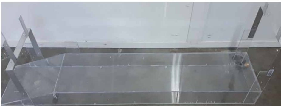
Figure 4. The lower reservoir, with the role of collecting the water drained through the intake orifices [55].
