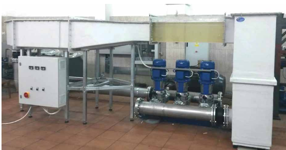
Figure 5. The experimental facility of the closed-circuit hydraulic stand [12].
