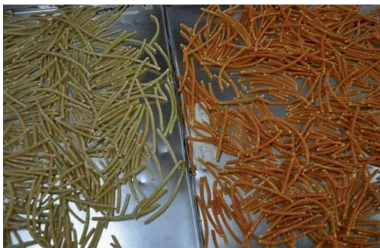
Figure 3. A detailed image featuring two varieties of dried extruded corn pellets, each with the same composition but different moisture content (the authors).
