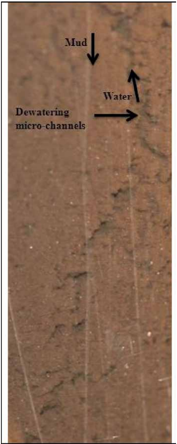
Figure 6. Photograph of a dewatering micro-channel in Lake Apopka mud. The mud is consolidating by expelling water sideways from the flocs, and this water flows upwards in the micro-channel.
