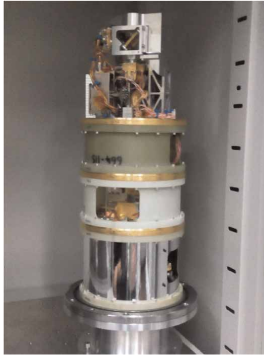
Figure 7. The band 8 receiver optics fitted into a self-contained cartridge for the ALMA telescope.
