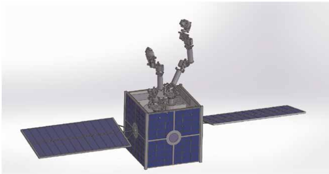
Figure 1. Conceptual representation of a multi-robot spacecraft system.
