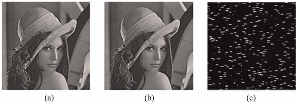
Figure 19. Transmission of a (512 \times 512) -pixel image between Alice and Bob at \text{SNR} = 0.1\text{dB} , with interception attempted by Eve [36]. (a) Original image transmitted by Alice using parameters \sigma = 10 , \rho = 54 , \beta = 4 . (b) Reconstructed image by Bob using recovered parameters \sigma = 10 , \rho = 54 , \beta = 4 and 0% pixel error. (c) Reconstructed image by Eve using incorrect parameters \sigma = 10 , \rho = 45.6 , \beta = 14 and 98.4652% pixel error.
