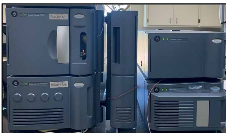
Figure 4. Waters™ Acquity high performance liquid chromatography system (top and bottom left) equipped with a column heater (middle) and coupled with a Waters™ 2998 PDA ultraviolet detector (top right) and Waters™ QDa mass spectrometer detector (bottom right).
