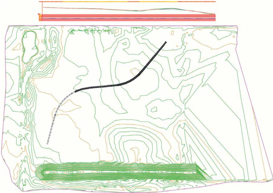
Figure 1. DTM, road alignment and its vertical profile.
