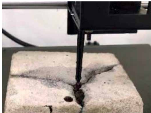
Figure 6. Automated 3D printing for pavement repair in concrete and asphalt.
