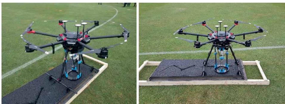
Figure 5. Leeds University's repair drone [13].
