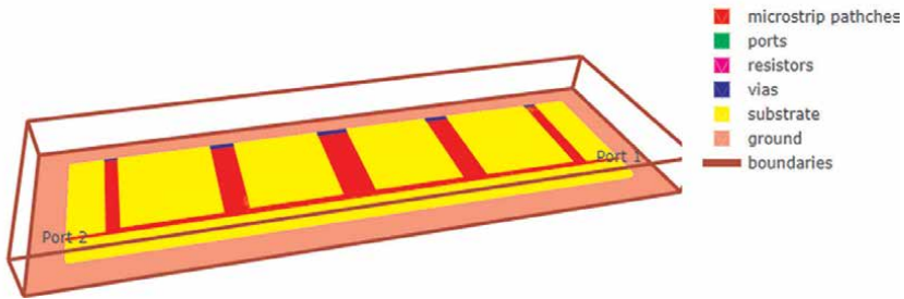
Figure 5. The geometry of a band pass filter presented in Hong [13].
