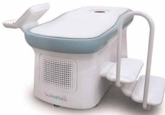
Figure 1. The Wavelia#2 microwave breast imaging prototype.
