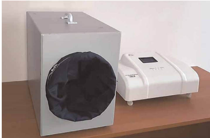
Figure 3. A design of the rewarming limb device with a microwave chamber and a generating unit of SMVI-200 medical physiotherapeutic device [16].
