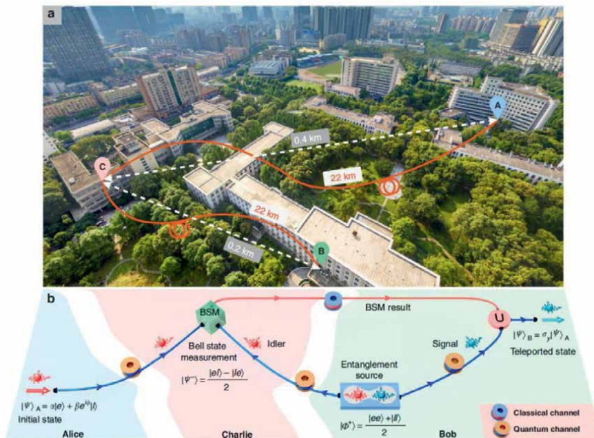
Figure 9. (a) Aerial view of the teleportation system based on UESTC backbone network. (b) Scheme of the teleportation system. From ref. [65] (reuse with approved CC BY license).
