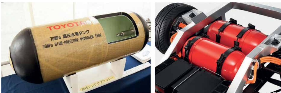
Figure 4. Hydrogen storage tank under 70 MPa pressure for the Toyota Mirai car and a hydrogen storage system in the Honda FCX Clarity car [10, 11].
