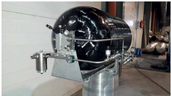
Figure 8. Examples of compressed hydrogen storage systems, A-35 MPa and B-70 MPa.
