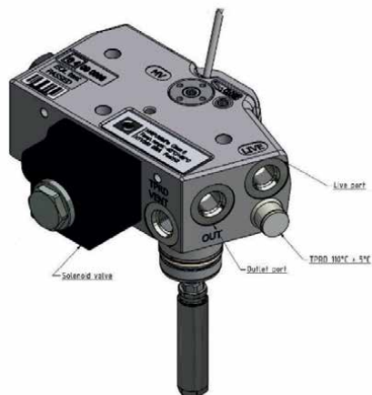
Figure 7. Sketch of the HTV 350 OMB Saleri operation valve for composite valve and its primary technical data.
