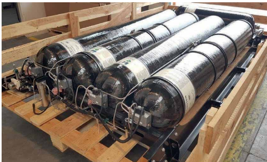
Figure 9. Compressed hydrogen storage system for a bus.
