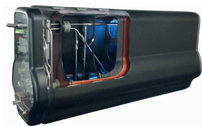
Figure 13. A tank developed by the BMW group for a hydrogen-powered car [20].
