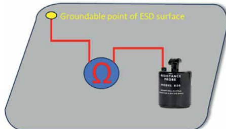
Figure 17. Resistance to groundable point measurement ( R_{gp} ).
