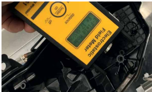
Figure 2. Charged housing of automotive headlight—measured 17.6 kV/m.
