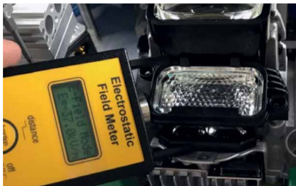
Figure 3. Charged plastic parts of automotive headlight with PCB installed—measured 37.0 kV/m on a PCB.
