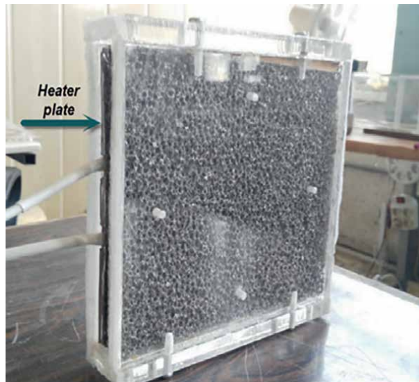
Figure 6. Single-cell metal foam adjacent to electrical heater plate [9].
