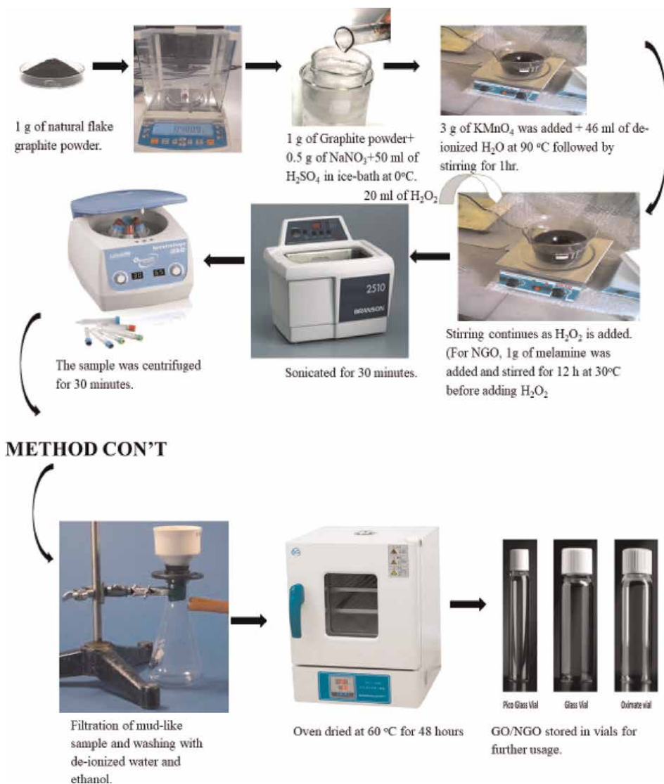
Figure 4. Synthesis procedure of graphene oxide (GO) and nitrogen-doped graphene oxide (NGO).
