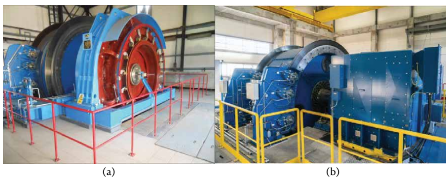
Figure 3. The winding machine with a DC motor (a) and a synchronous motor (b). [SIEMAG TECBERG POLSKA].
