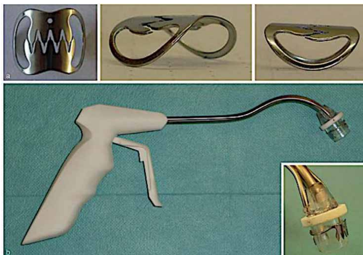
Figure 11. Over the scope clip (OTSC) equipment. (a) Representation of the “bear claw” clip that is deployed and (b) the OTSC proctology device. Reused from Prosst et al. [119] with permissions from Taylor and Francis.
