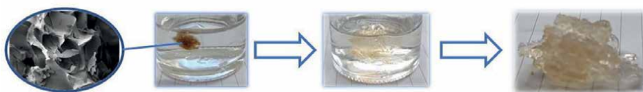
Figure 2. SEM image of PEG doped superabsorbent polymer and its swelling in water over time [71].
