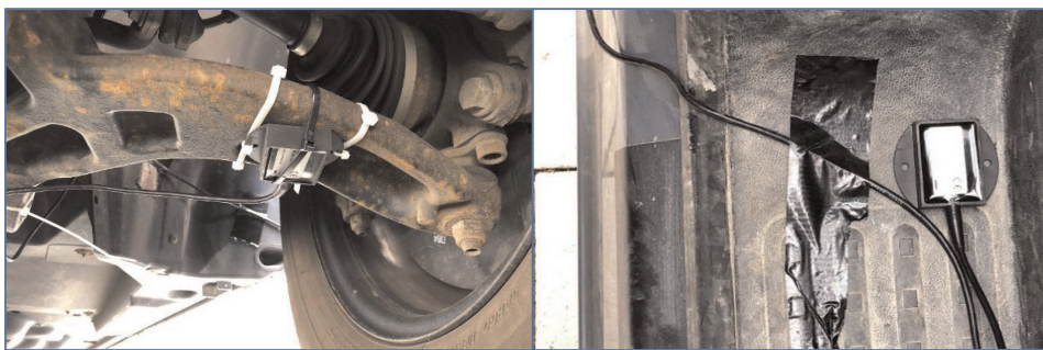
Figure 5. Sensor under wheel carrier (left) and sensor in vehicle interior (right) [5].
