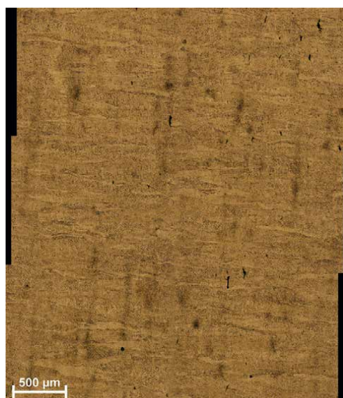
Figure 13. Optical microscopy image of the microstructure of the Ti-6Al-4V alloy, obtained by additive manufacturing printed in the Z-direction.
