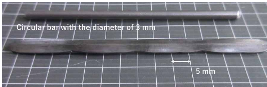
Figure 20. An incremental shaping with r = 45\% to continuously deform the round bar to a triangular cross-section bar by shifting the CS-punch in each 20 mm.
