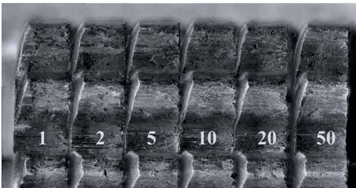
Figure 27. Continuous fine blanking of pure titanium gears up to N = 50 . The gear side surface condition was improved with increasing N .
