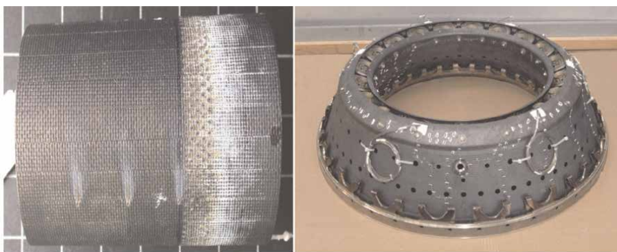
Figure 1. CERASEP®A415 rig and inner & outer liners of an engine combustor [7].
