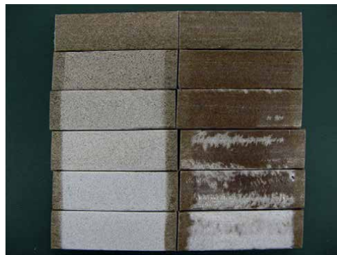
Figure 5. Discoloration of uncapped WPCs (left column) and Co-WPCs (right column) after various weathering times (0, 192, 432, 744, 1392, and 1952 h) [4].
