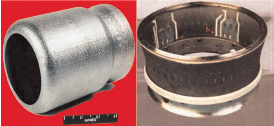
Figure 2. CMC combustor liner by GE and Allison [8].
