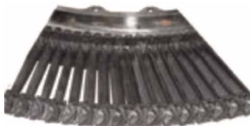
Figure 12. Cerasep® A40C low-pressure turbine blade developed by Herakles [20].
