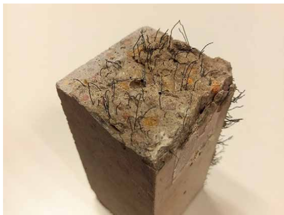
Figure 1. Cracking surface of a steel fiber-reinforced concrete specimen.
