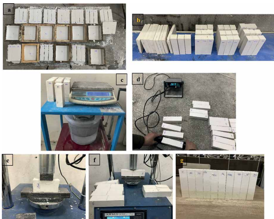
Figure 2. Images of experimental procedure. (a) Samples in molds, (b) all samples, (c) apparent porosity test, (d) ultrasonic pulse velocity test, (e) compressive strength test, (f) bending strength test, (g) capillary water absorbed samples.
