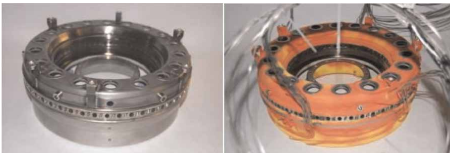
Figure 4. MI SiC/SiC combustor before and after rig test [10].
