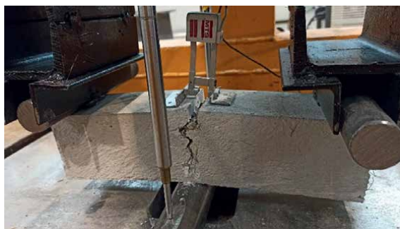
Figure 5. Three-point bending test on the SFRC specimen. The final phase in fully cracked state.
