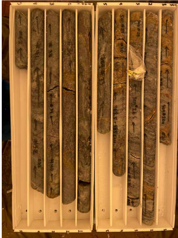
Figure 15. Subglacial rock core from the ASIG drilling at Prudhoe dome (photo credit: Allie Balter-Kennedy).
