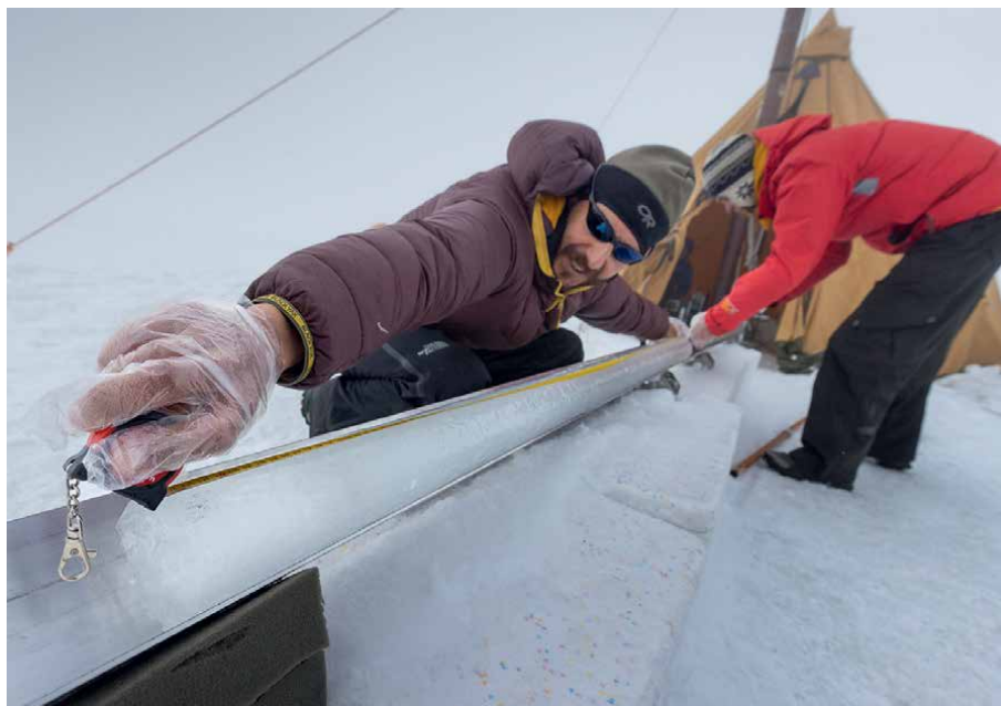
Figure 7. The science team measures and processes an ice core drilled on Quelccaya (photo credit: Mariusz Potocki).
