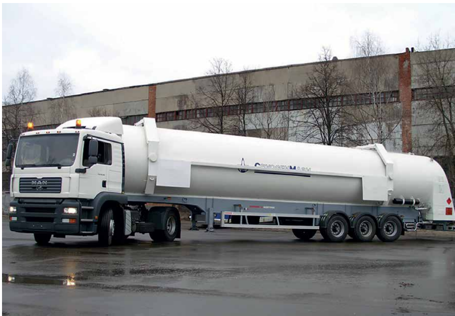
Figure 6. Automobile tank of JSC “Cryogenmash” for liquid hydrogen transportation [37].
