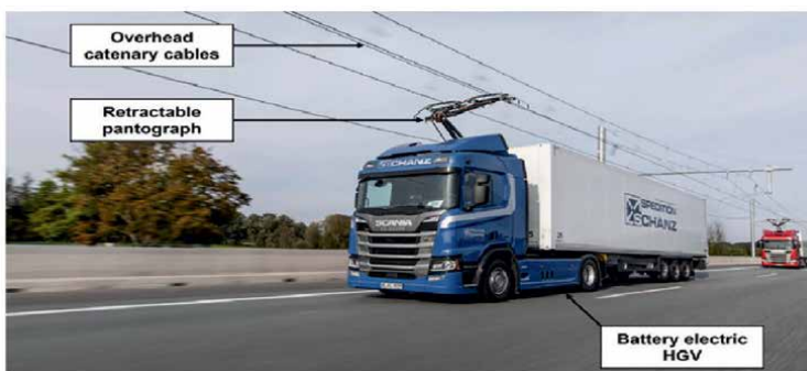
Figure 4. An overhead catenary implementation of ERS. Source: Siemens Mobility GmbH, 2022, as cited in [19].
