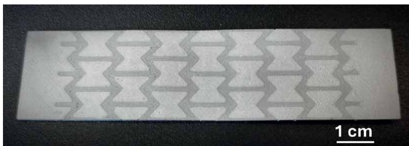
Figure 12. Sintered part combining 17-4PH (dark gray) and 316L (light gray) stainless steels, designed with a pattern to enhance the overall properties of the part. Dimensions: 75 cm × 2.5 cm × 1.5 mm thickness.
