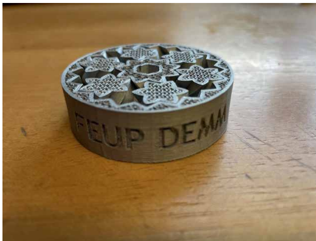
Figure 5. Gear bearing optimized with lattice structures.
