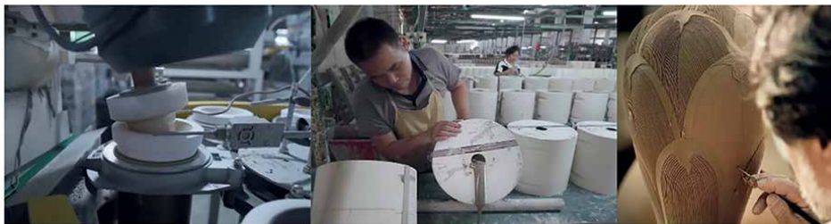
Figure 4. Industrial machine ceramic body (left), mold casting ceramic body (middle), hand-carved details of the ceramic body (right).
