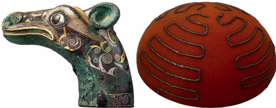
Figure 3. Horse-head-shaped bronze chariot ornament inlaid with gold and silver; warring states period (403–221 BC), collected in the National Museum of China (left) and curved nano-silver antennas fabricated by FDM and DIW printing techniques (right).
