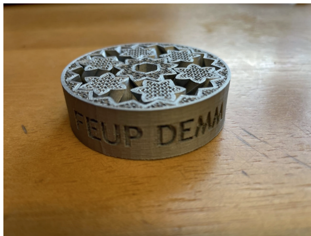
Figure 5. Gear bearing optimized with lattice structures.
