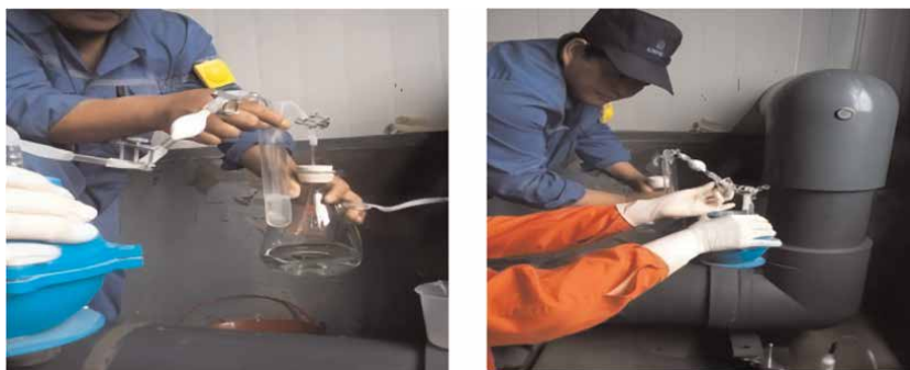
Figure 5. Gas and radon sampling site of infusion tub device.
