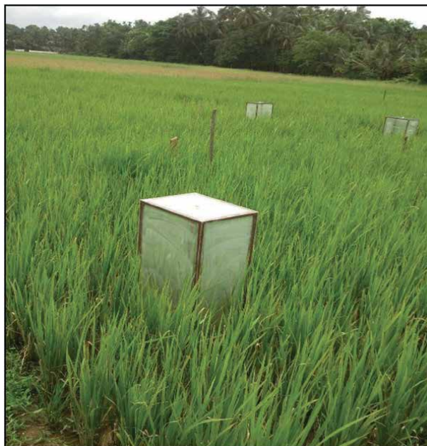
Figure 4. Box chamber with hills placed in the field for GHG collection.
