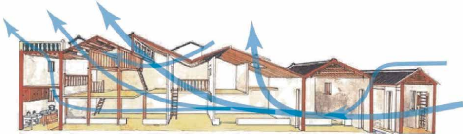
Figure 7. Space design in Lingnan for natural ventilation.
