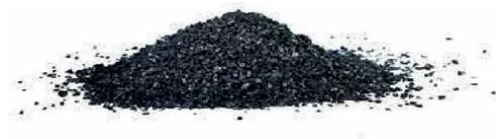
Figure 9. Activated carbon particles (source: [97]).
