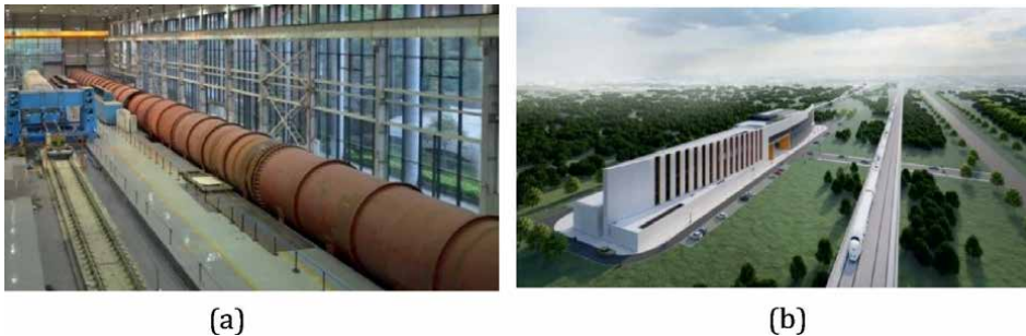
Figure 20. Evacuated tube HTS Maglev test platform. (a) 140 m long evacuated tube [35]. (b) Multimodal coupled rail transit moving model test platform [36].
