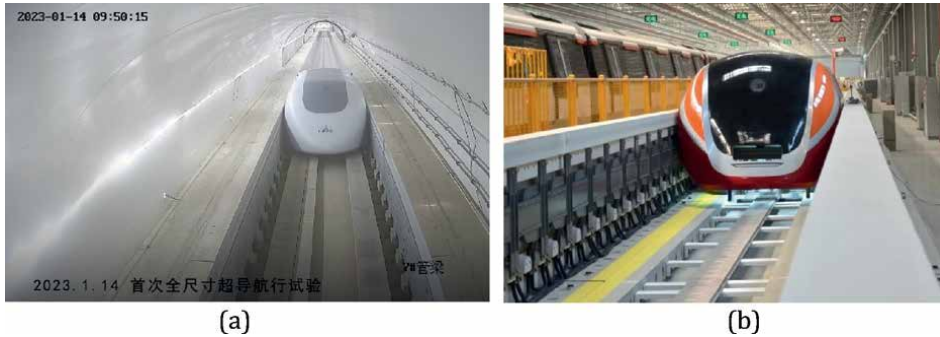
Figure 13. Superconducting EDS principal prototype in China. (a) CASIC's HTS EDS test [24]. (b) CRRC Changchun's HTS EDS test system [25].
