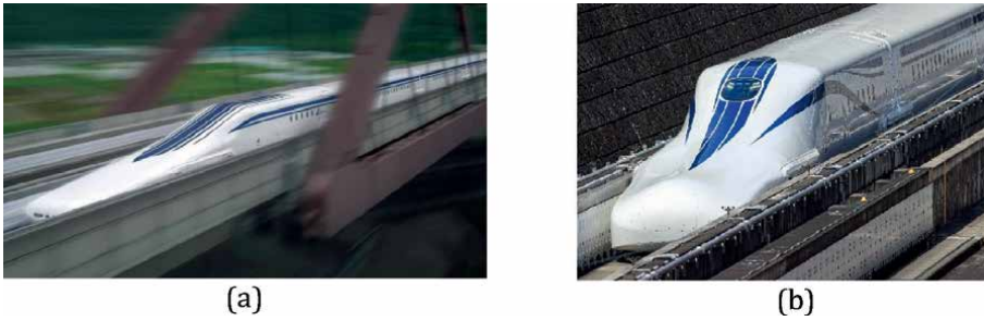
Figure 11. Superconducting EDS train on Yamanashi test line in Japan [20]. (a) Series Lo Version. (b) Series Lo Improved Version.
