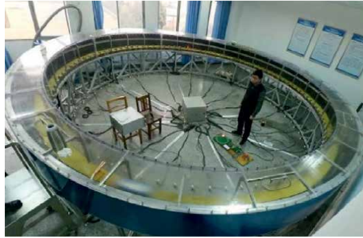
Figure 19. Side-suspended HTS Maglev circular test track system [34].
