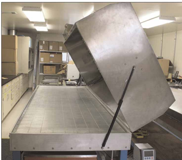
Figure 1. Thermal gradient table used to determine optimum crop seedling growth over time (photograph by Sidney Cromer).
