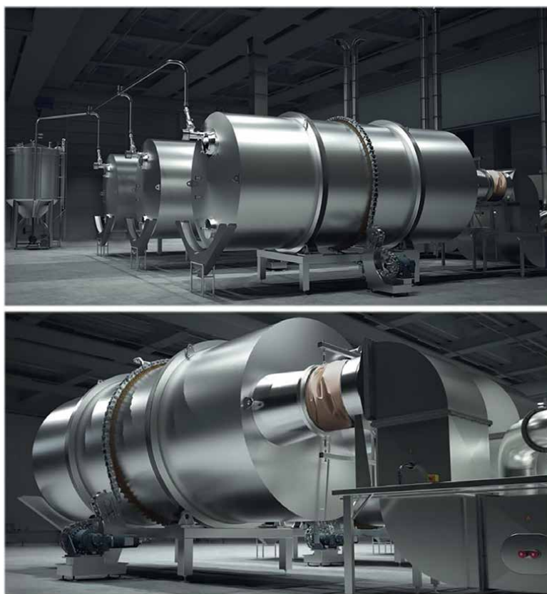
Figure 7. The SCHULZ malting system's germination-kilning combo drum Kaspar Schulz | Malting in detail ( kaspar-schulz.de ).
