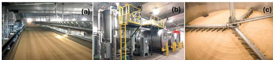
Figure 2. (a) Malting in a large open germinating box (ukmalt.com), (b) steeping tank and drum-style system (maltersadvantage.com), and (c) grains in steeping tank (https://canadamalting.com/process/).
