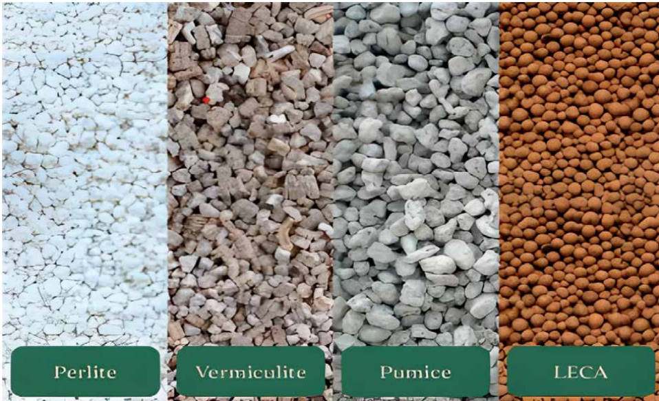
Figure 1. Inert substrates in hydroponic farming systems. This figure shows common inert substrates like perlite, vermiculite, pumice, and LECA, used in hydroponic systems for their excellent aeration, drainage, and non-reactive properties, which support healthy root growth and stable nutrient conditions. Source: Olympios [9].
