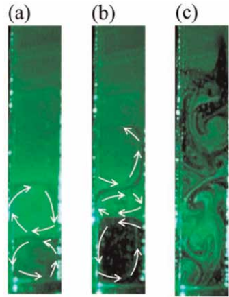
Figure 6. Observed vortices at each stage in Case II ( Re = 496 , Gr = 8.8 \times 10^7 ): (a) stable Taylor vortices, (b) deformed Taylor vortices, and (c) collapsed Taylor vortices [20]. Arrows in figures denote the vortex motion.
