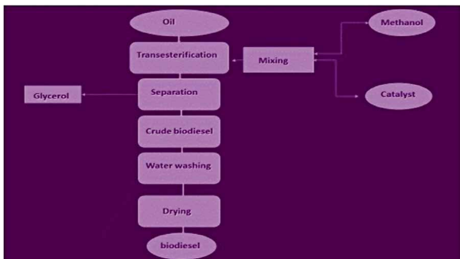
Figure 1. Schematic flowsheet of the transesterification process for biodiesel production.
