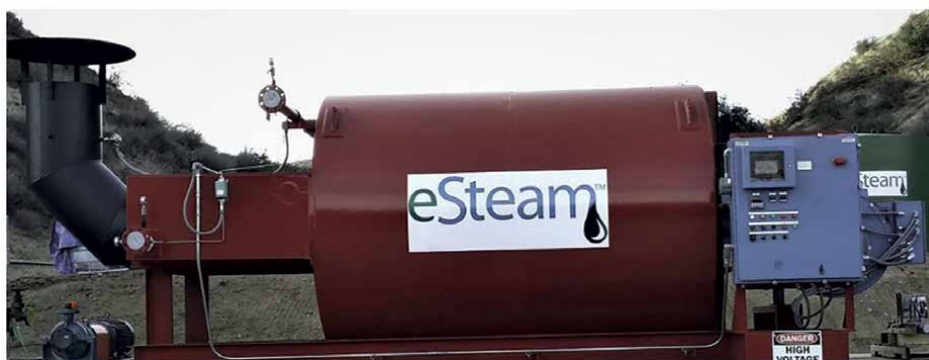
Figure 5. 8 MMBtu/hr. thermal fluid heater. Source: www.esteamoil.com .
