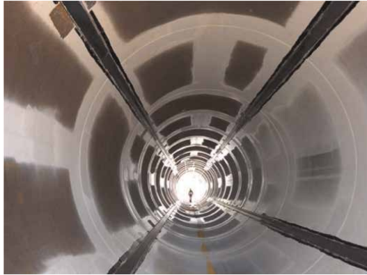
Figure 5. Location of optical fibers with FBGs on the inside of an instrumented monopile [2].
