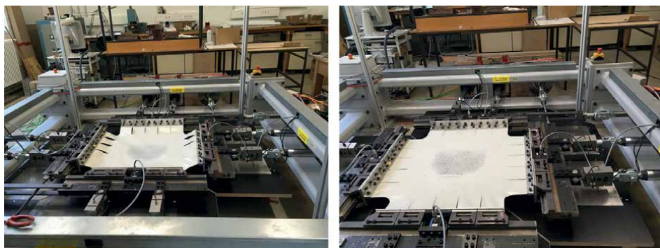
Figure 15. Biaxial testing equipment, unloaded (left) and loaded (right) [© Rosemarie Wagner].
