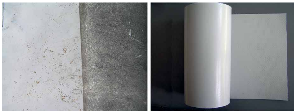
Figure 12. Inside and outside of an approx. 5-year-old cover (left), PVC coating with PVDF layer on one side (right) [© Rosemarie Wagner].
