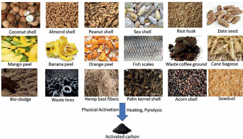
Figure 2. Synthesis of BAC from biomass via physical activation.
