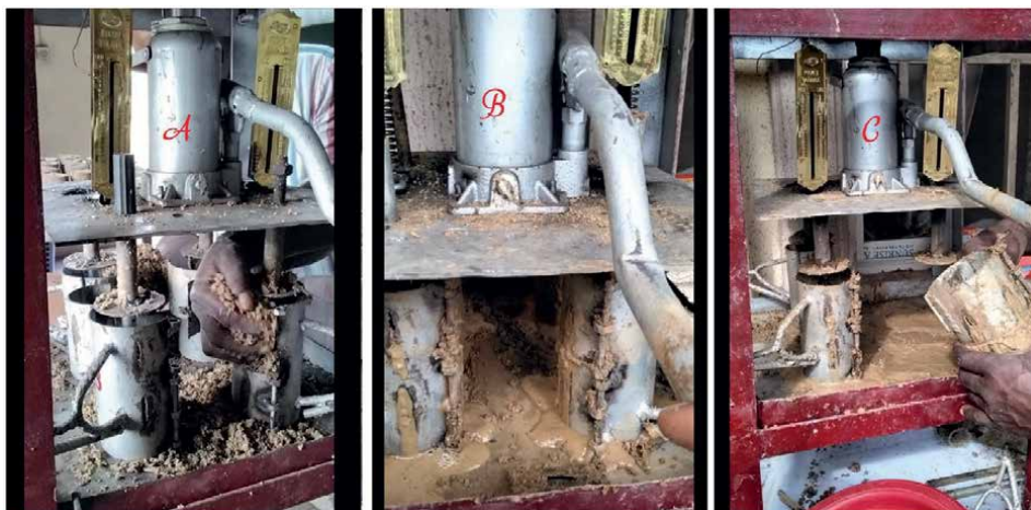
Figure 3. The developed hydraulic briquetting machine and production. A. Material loading, B. Material compression, C. Removing mold.
