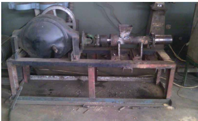
Figure 2. Existing experimental screw press extruder.
