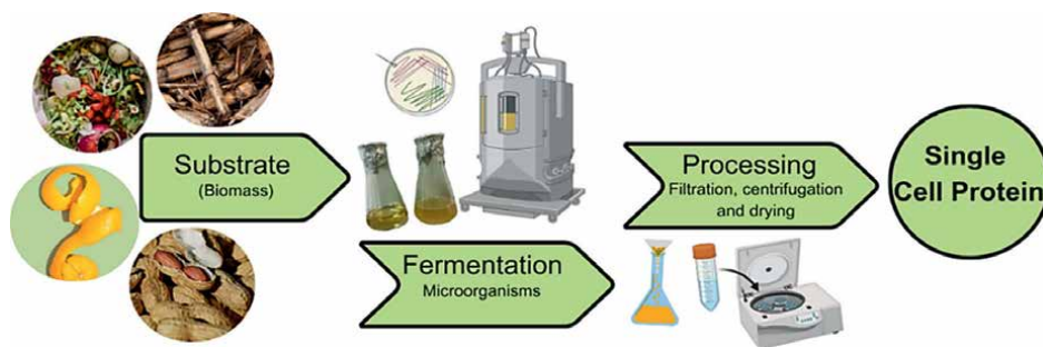
Figure 2. Schematic illustration of the SCP production process.
