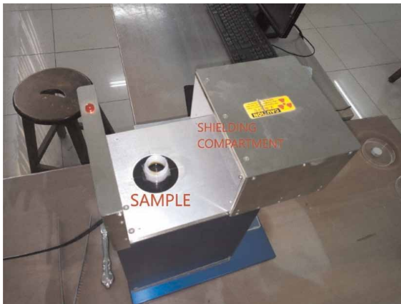
Figure 7. Sample holder inside the AMPTEK shielding compartment EXP 1 X-123 XRF Experimenter Kit displaying the detector for the sample arrangement.
