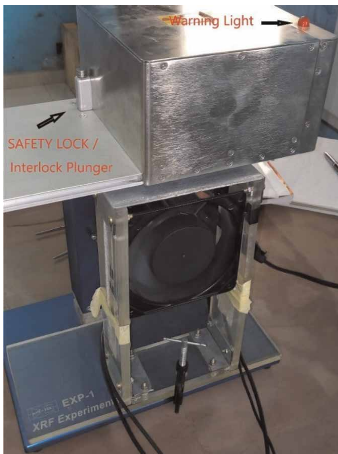
Figure 8. The safety plunger-equipped shielding section displaying the AMPTEK EXP 1 X-123 XRF experimenter's safety features set.
