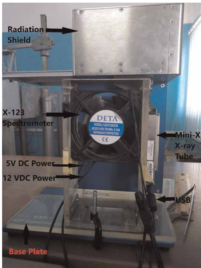
Figure 6. Kit for AMPTEK EXP-1 X-123 XRF experimentation displaying the Mini-X-ray tube radiation source and spectrometer (X-123) both located below the container for radiation protection.
