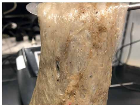
Gel damage from friction reducing “SLICK WATER” additives
