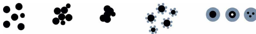
Figure 1. Particles in dispersions. From left to right: monodispersed nanoparticles, agglomerates, aggregates, surface functionalized nanoparticles, core-shell nanoparticles (images are not to scale).
