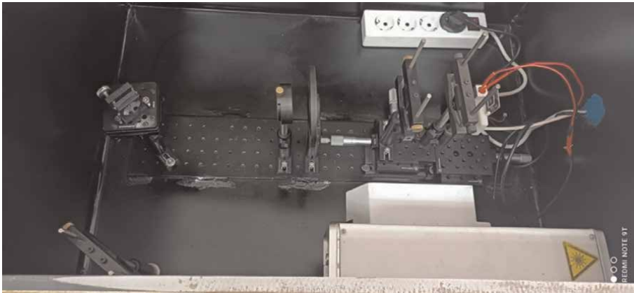
Figure 5. Beam displacement experimental setup.
