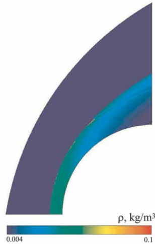
Figure 8. Density contours computed with the Roe scheme and inviscid model.
