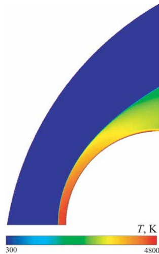
Figure 13. Temperature contours computed with equilibrium chemical reactions in high-temperature air.
