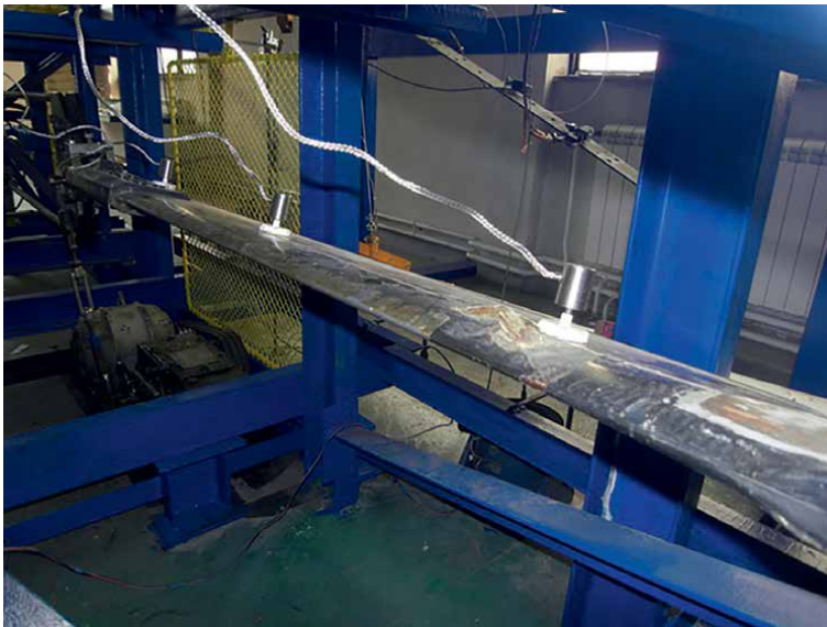
Figure 24. Position of the accelerometers.
