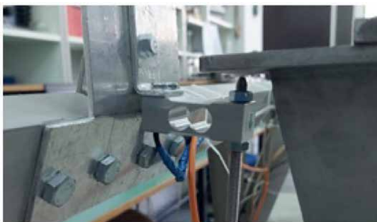
Figure 2. Thrust measurement setup.
