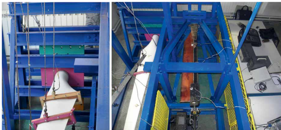
Figure 8. Acceptance and mounting of the blades for rigidity testing (left) and fatigue testing (right).
