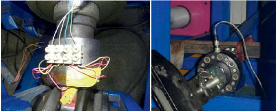
Figure 23. Integrated strain gauges (left) and reference force transducer (right).
