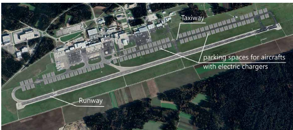
Figure 1. Airport with additional 85 parking spaces with electric chargers for electric planes along the taxiway (Airport Ljubljana).
