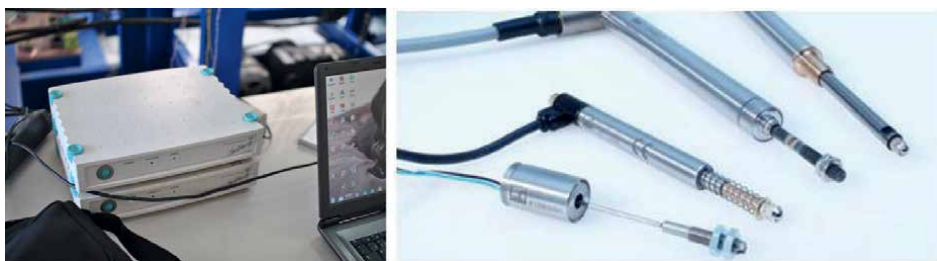
Figure 12. Two modules of SPIDER 8 and inductive displacement sensor LVDT—HBM.
