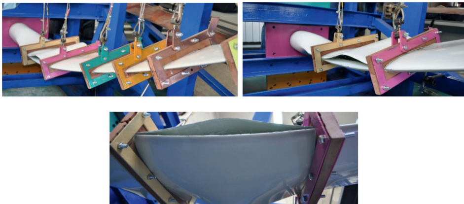
Figure 17. Position of the blade fracture.
