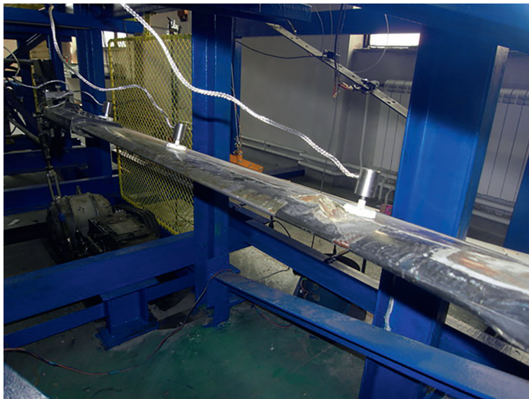
Figure 24. Position of the accelerometers.
