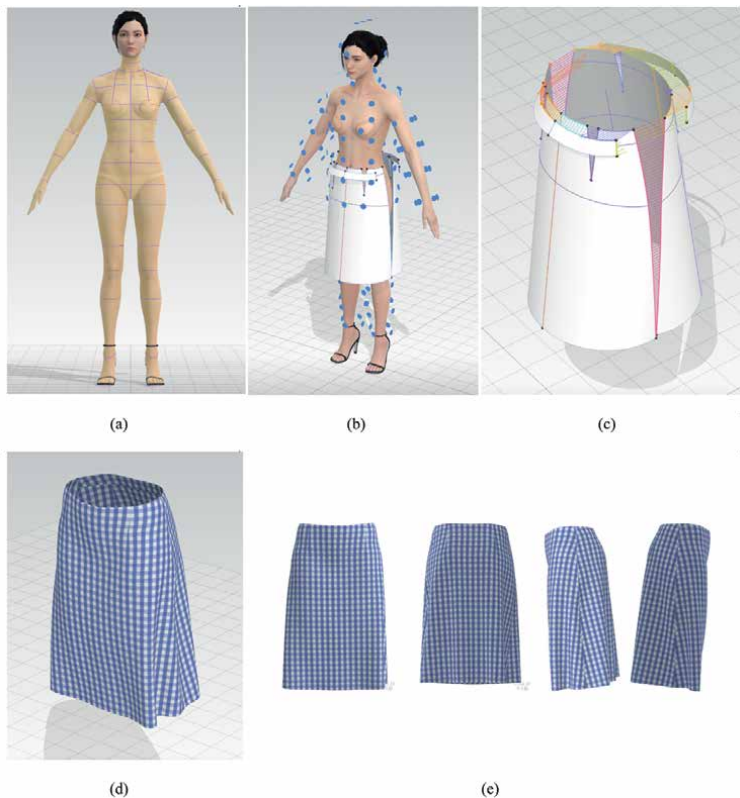
Figure 6. Basic steps to generate a DTCA in Style3D: (a) avatar selection and editing with body dimensions, (b) arrangement of 3D PB, (c) arrangement of virtual sewing threads, (d) TM texture and physical properties editing, (e) export of the apparel.
