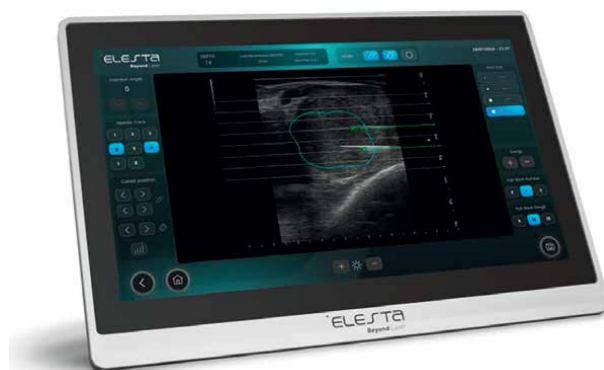
Figure 2. The Echolaser smart interface (ESI).
