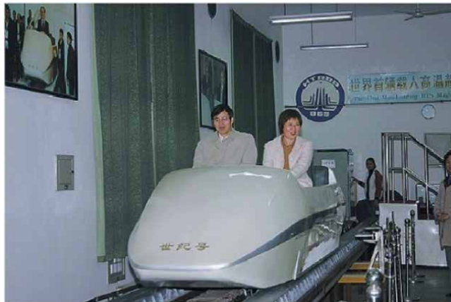
Figure 10. The world's first manned high-temperature superconducting pinning suspension car.
