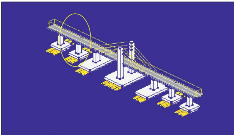
Figure 3. Distributed impact loads along the build model.
