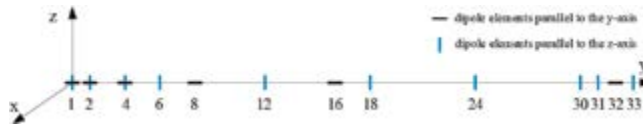
Figure 1. Sparse polarimetric array composed of 6 NA dipoles (axial directions parallel to the y-axis) and 10 ANA dipoles (axial directions parallel to the z-axis).
