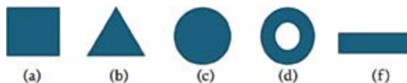
Figure 3. Microstrip antenna types and shapes (a) Square, (b) Triangle, (c) Circle, (d) Ring, and (e) Dipole.
