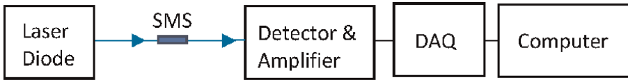
Figure 5. Block diagram of an MMI temporal measurement setup. DAQ stands for data acquisition system.
