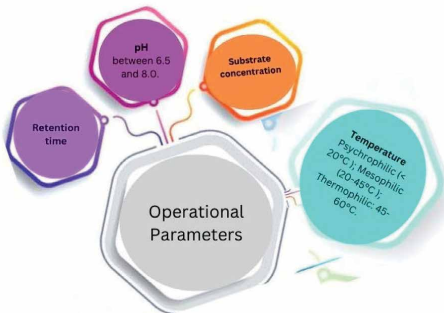
Figure 2. Factors that influence anaerobic digestion.
