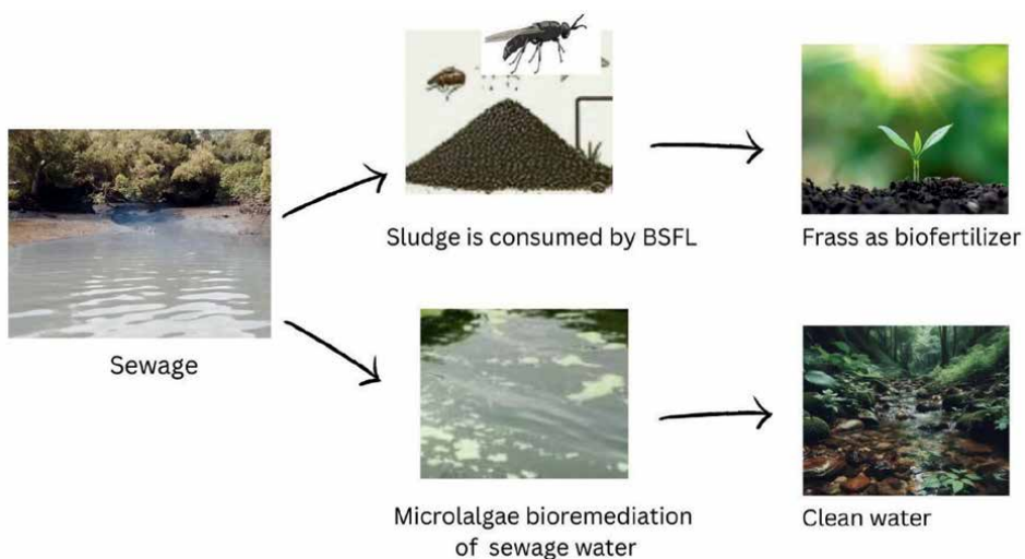
Figure 2. Proposed set-up for sewage treatment using BSFL and microalgae.
