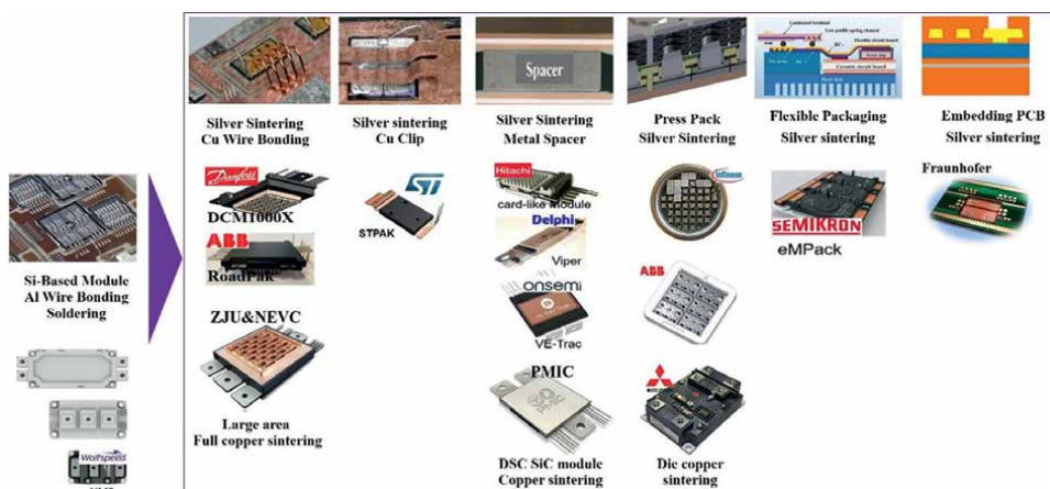
Figure 9. Module packaging architecture transition from Si-based IGBT to SiC MOSFETs.
